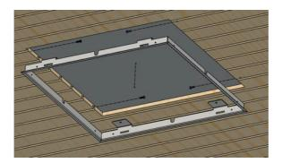
3. Slide the heating element into the mounting frame until the protruding tabs are locked in place.
