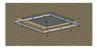
2. Variant no.2 Fixing to recess Fix the tabs to the recess
